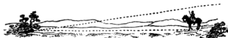
FIG. 4.—MISSING THE ENEMY THE SOLDIER LYING DOWN IS SUPPOSED TO HAVE SET THE SIGHT OF HIS GUN FOR A RANGE OF 1000 YARDS BY MISTAKE, AND WHEN HE AIMS AT THE CAVALRYMAN, WHO IS ONLY A SHORT DISTANCE AWAY, THE BULLET GOES RIGHT OVER THE CAVALRYMAN'S HEAD, AS IS EXPLAINED IN THE CHAPTER.
