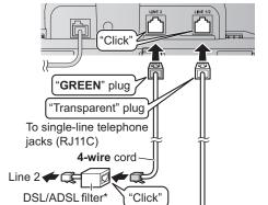
\*DSL/ADSL filter (not supplied) is required if you have DSL/ADSL service.
