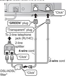
\*DSL/ADSL filter (not supplied) is required if you have DSL/ADSL service.
