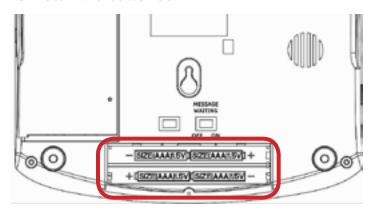
Battery compartment on the bottom of the phone
