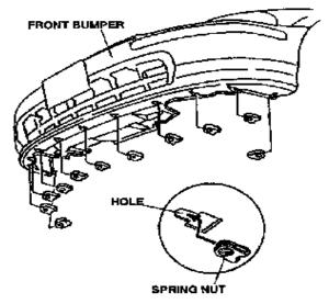
Position the chin spoller on the front bumper, and loosely install the two flange bolts and nine bumper bolts as shown.
