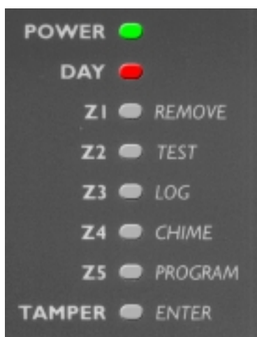
The system is Unset (Day Mode) Only PA and Tampers are active
