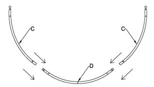
Slide the ends of the upper section (C) over the ends of the bottom of the upper section (D) Do not bolt together.
