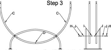
Attach the upper sections (C and D) to the inside of the bottom section (A) using the  $\frac{3}{8}$  bolts, washers, and nuts. Place the bolts and washers on the outside with the nuts inside. These bolts will connect section C to section D as well as the entire upper unit to the bottom section (A).
