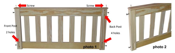
**Step 2:** Insert two dowel nuts in the holes in each end of the bottom backrest board and on the inside of the front rail. Push them in all the way and turn so the threaded holes align with the holes in the ends of the rails. (See photos 3, 4 & 5).
