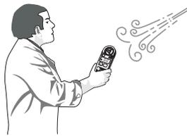
The Kestrel turns itself off automatically after 30 minutes of no button presses.
